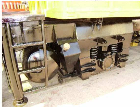
Fig. 4. Measuring no. 32 [6] Braking distance and pressures in braking installation Fig. 5 Axle bearing on which the encoder is installed.
