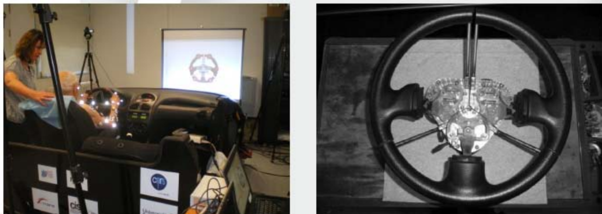
Figure 5a (left): Experimental device to study the steering movement for disabled people. Figure 5b (right): Instrumented steering wheel with three dynamometers.
