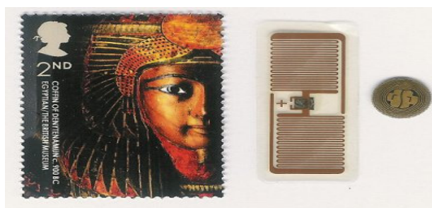
Figure 5 RFID chips that can be integrated into the postage stamp
