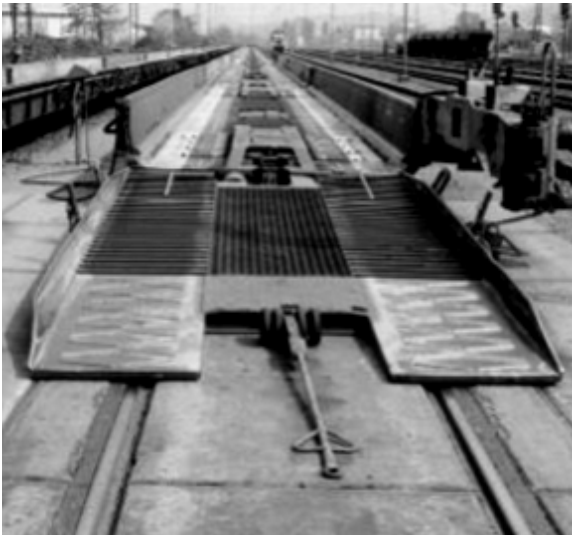
Figure 3. Frontal ramp for reloading road freight vehicles
