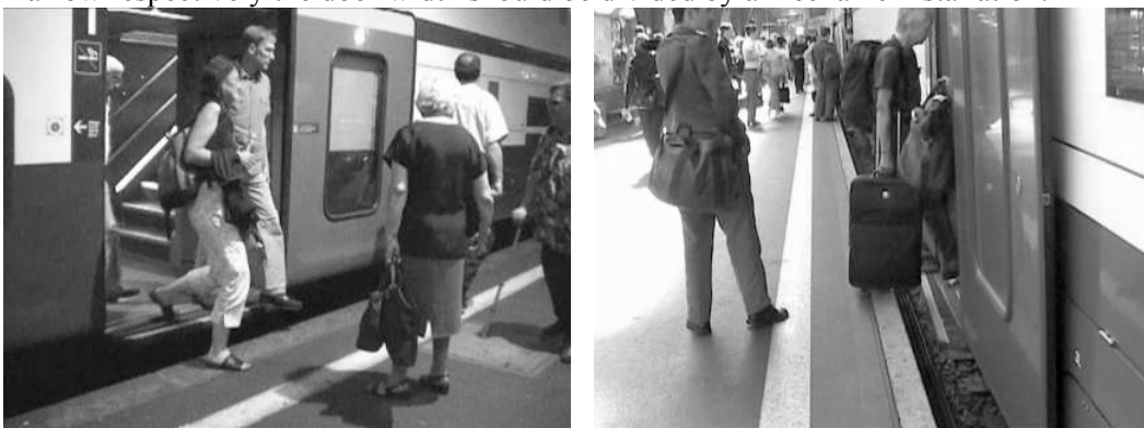
Fig.6 IC2000 on a platform height of 38cm (left) IC 2000 on a platform height of 55cm (right)
