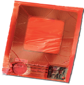
Figure 1 RFID post tag for the postal test letters (IPC 2011)
