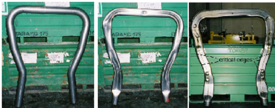
Fig.4 Bending, pre-forming and hydroforming of steel profiles (TATA STEEL)
