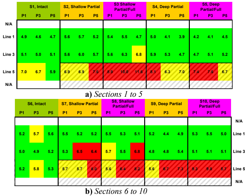
Fig. 6 Statistical Analysis of FWD Deflection on Small Scale Study
