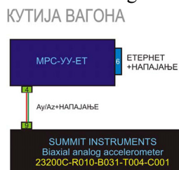
Fig.10 Block diagram of the measuring system for measurement of acceleration of the wagon body
